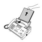
2 Open the operation panel (grasp the finger hold and pull up), and then pull the release on the right side of the machine forward to open the print compartment cover.
